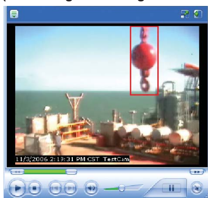
FIGURE 1 Video of a Production Platform (with Intelligent Tracking of a Crane)
