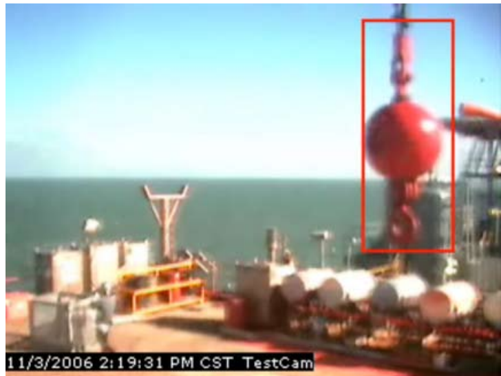
Figure 3: Smart digital cameras and video analytics software can detect and track an intruder. Here, a camera on an offshore platform spotted a crane hook moving across its field of view, put a red box around it, and tracked the hook until it disappeared from view.
