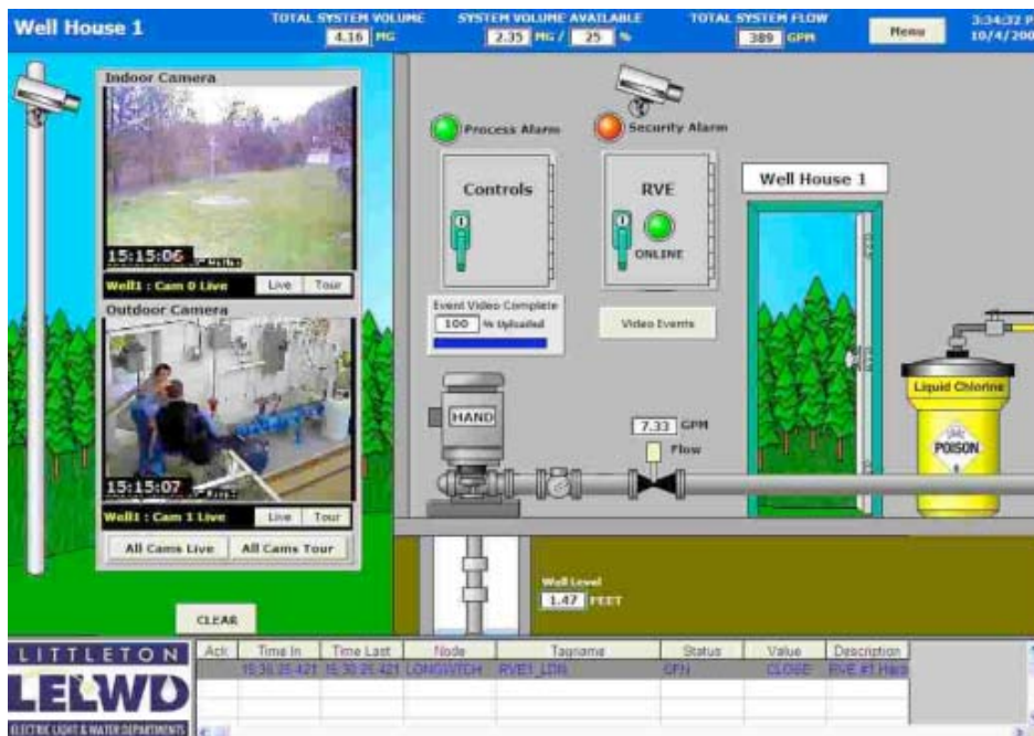
Figure 1: Water treatment plants pioneered the use of video in HMI/SCADA systems. Here, a water plant in the U.S., displays video clips transmitted over the plant's industrial network on a Wonderware HMI system.
